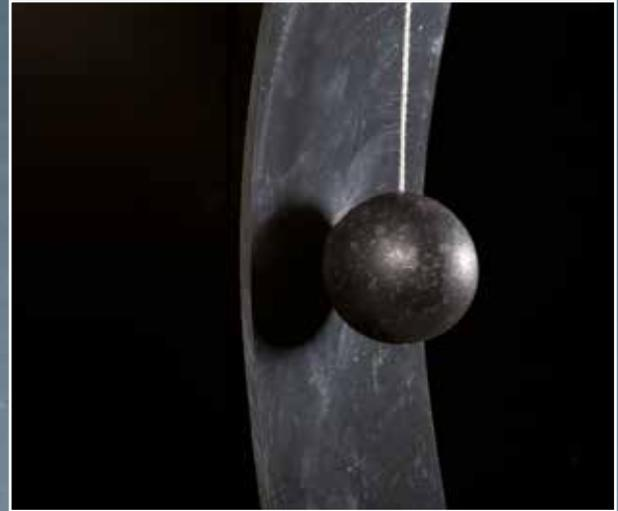
These pictures show that RECYFIX withstands the impact of a hurled steel ball. Here it proves its characteristics of flexibility, toughness and unbreakability.
