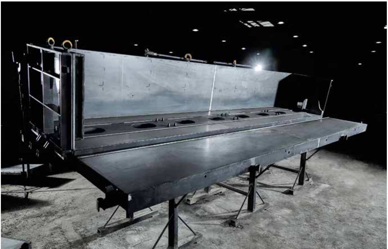
Mould for the production of a 4-metre TRAFFIC GUGI®BLOC+ section
