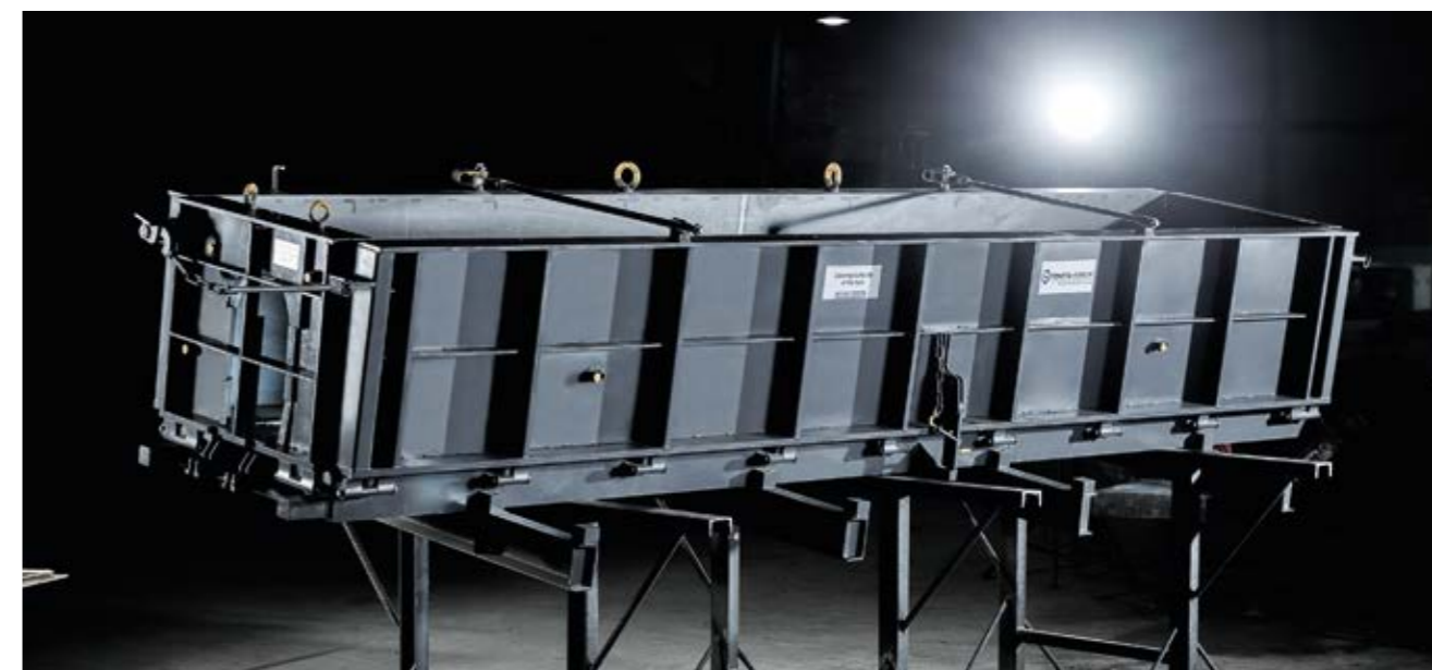
Form for the production of a 4-metre section of TRAFFIC GUGI®BLOC+
