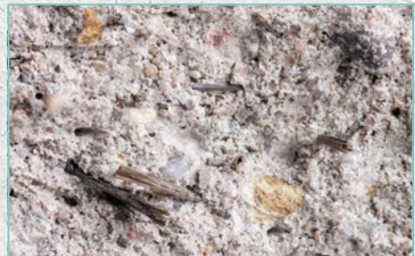
Macro view of FASERFIX concrete. The fibres that give the material its high strength are clearly visible.
