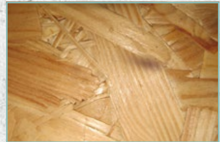
Wood fibre boards get their high stability from a densely woven fibre network.
