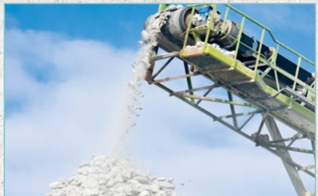
Concrete recycling, re-use e.g. in road construction.
