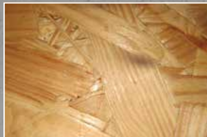
Wood fibre boards get their high stability from a densely woven fibre network.
