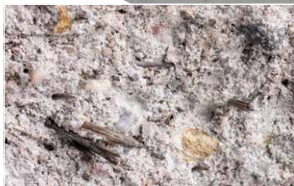
Macro view of FASERFIX concrete. The fibres that give the material its high strength are clearly visible.
