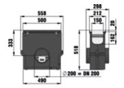
Trash box with plastic bucket, with ductile iron grating, black, SW 18 mm,
