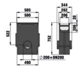
Trash box with plastic bucket, with ductile iron grating, black, SW 18 mm, class F 600, 4 holts fixing
