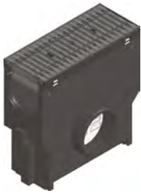
Trash box with galvanised mud bucket and FIBRETEC slotted grating, black, SW 9 mm, cl. B 125, locked
